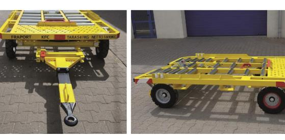
ca. 3200 mm Overall length (drawbar at the bottom) ca. 3920 mm Width 1680 mm Height ca. 500 mm Height (upper edge oft the idler) ca. 518 mm +/- 4mm Loading area (between stops) ca. 1545 mm / 1200 mm Length ca. 2495 mm Wheelbase ca. 1650 mm Ground clearance ca. 180 mm smallest turning circle diameter. (outside) ca. 3500 mm max. travel speed ca. 25 km/h Payload 1800 kg Dead load ca. 549 kg
